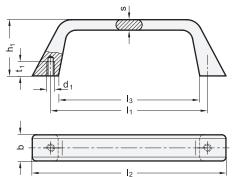
Drilling for cap screw DIN 912
